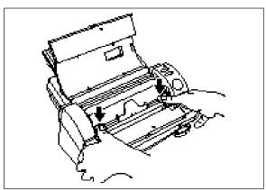
(5) Return the roller holder to the original position and press the roller holder lock buttons (purple color) as illustrated. You will hear the roller holder click into place. Press the roller holder further to secure the roller unit.
